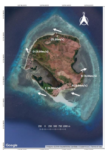
Fig 6. The velocity of longshore current at different points of Manamoc Island. Shown inside the red circle was the uneven seabed of the northwest beach indicating the difference in water depth. The map was generated using QGIS. Base map from Google Earth.
